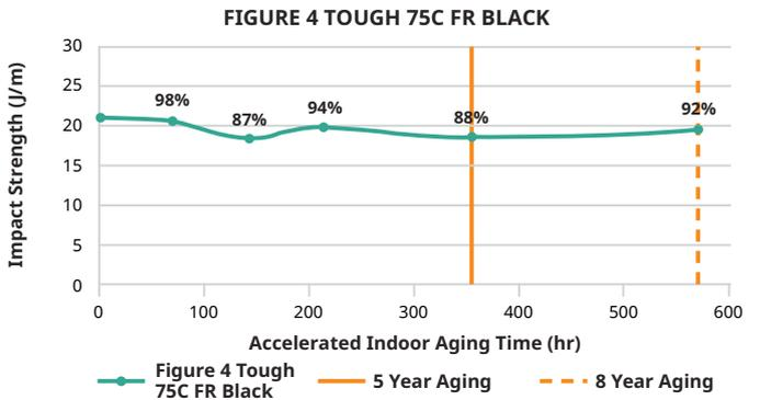
**OUTDOOR STABILITY:** Tested per ASTM G154 standard method.
