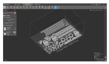
3D Sprint® software facilitates a streamlined and optimized transition from file to 3D print.
