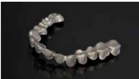
Metal dental pieces are taken from the ProJet 100 dental printer to have supports removed. Then they can have the surfaces finished so they're ready for use.
